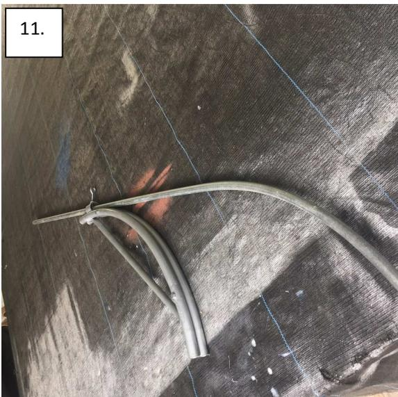
Flip the tubing end for end (change ends) and slide the other end through the clamp, stopping at the prescribed distance as for your model on the other end of tubing.
