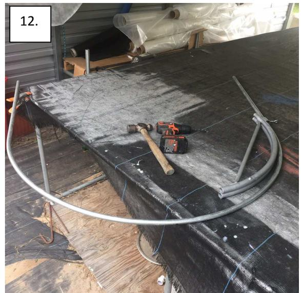
The completed hoop is still in the bender. This one was bent on our LT-4 bender. However the bending steps are always the same except the distance from the end you start bending.
