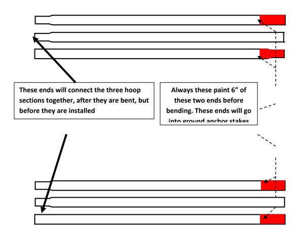
"D" Using factory 21 ft. lengths 1 3/8" 17 or 16 ga. cut in half.
