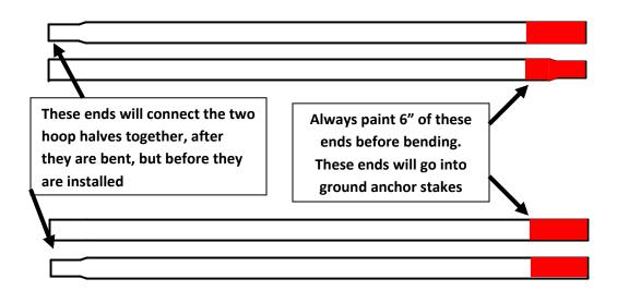
"B" Using factory 21 ft. lengths 1 3/8" 18 or 17 ga. cut in half.
