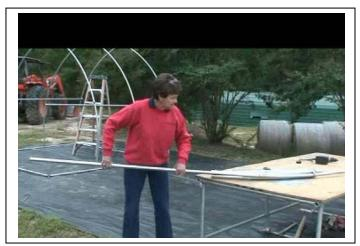
Repeat this step pulling and pushing about half of each bending stroke through the holding strap, add the lever bar (supplied) when needed for leverage.
